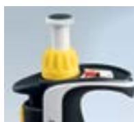
Red recalibration flag indicates adjustment from factory specifications.
