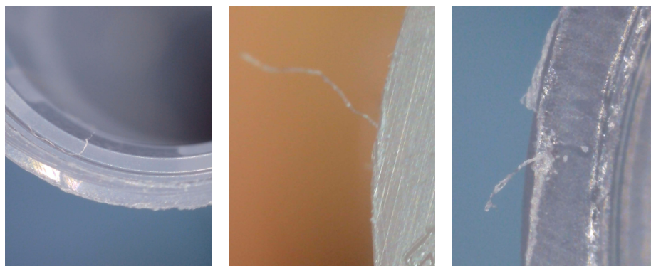
Figure 2. Stray fibers found in various, new, out-of-the-box (non-BRAND) pipette tips
