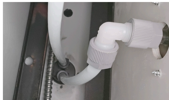
Tubing installed within a fume hood showing the connection fittings.
