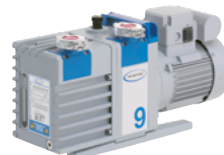
RZ9 2 \times 10^{-3} mbar, 165lpm Medium sized freeze-dryers
